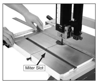
Figure 23. Squaring miter slot to blade.
